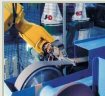
This dual-robot cell processes seven different styles of forged, near-net-shape connecting rods at up to 400 parts per hour. 14 surfaces and bosses are ground.
