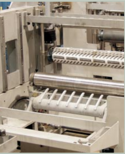
Breaker Roll flattens the strip against the Billy Roll, ensuring the material is level for grinding. The Breaker Roll can increase the amount of material wrap around on the Billy Roll.
