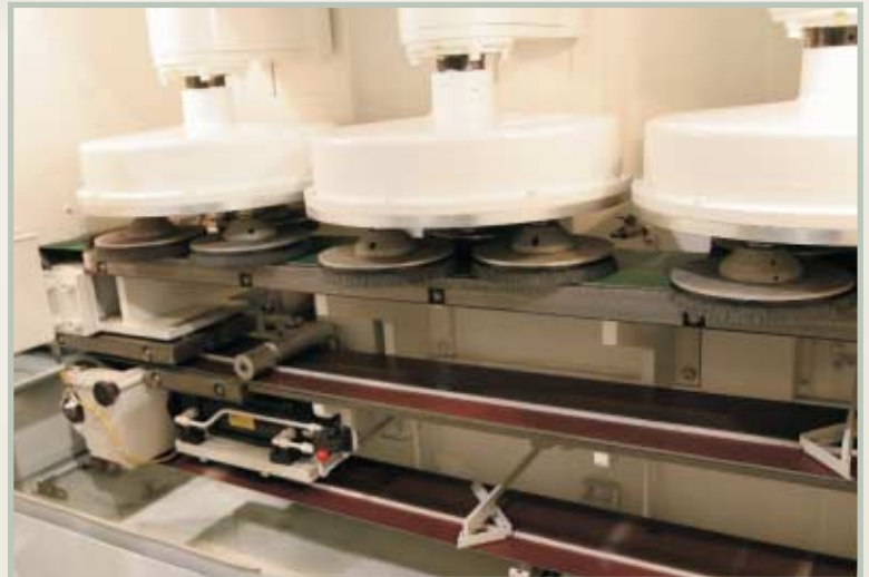
Triple-spindle planetary disc brushes (10 in. OD) deburr various automotive flat parts.
