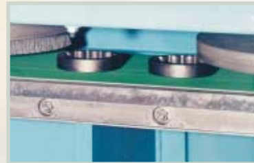
Planetary disc brush deburring is performed at 1500-2000 parts per hour on this Acme magnetic over/under conveyor system.
